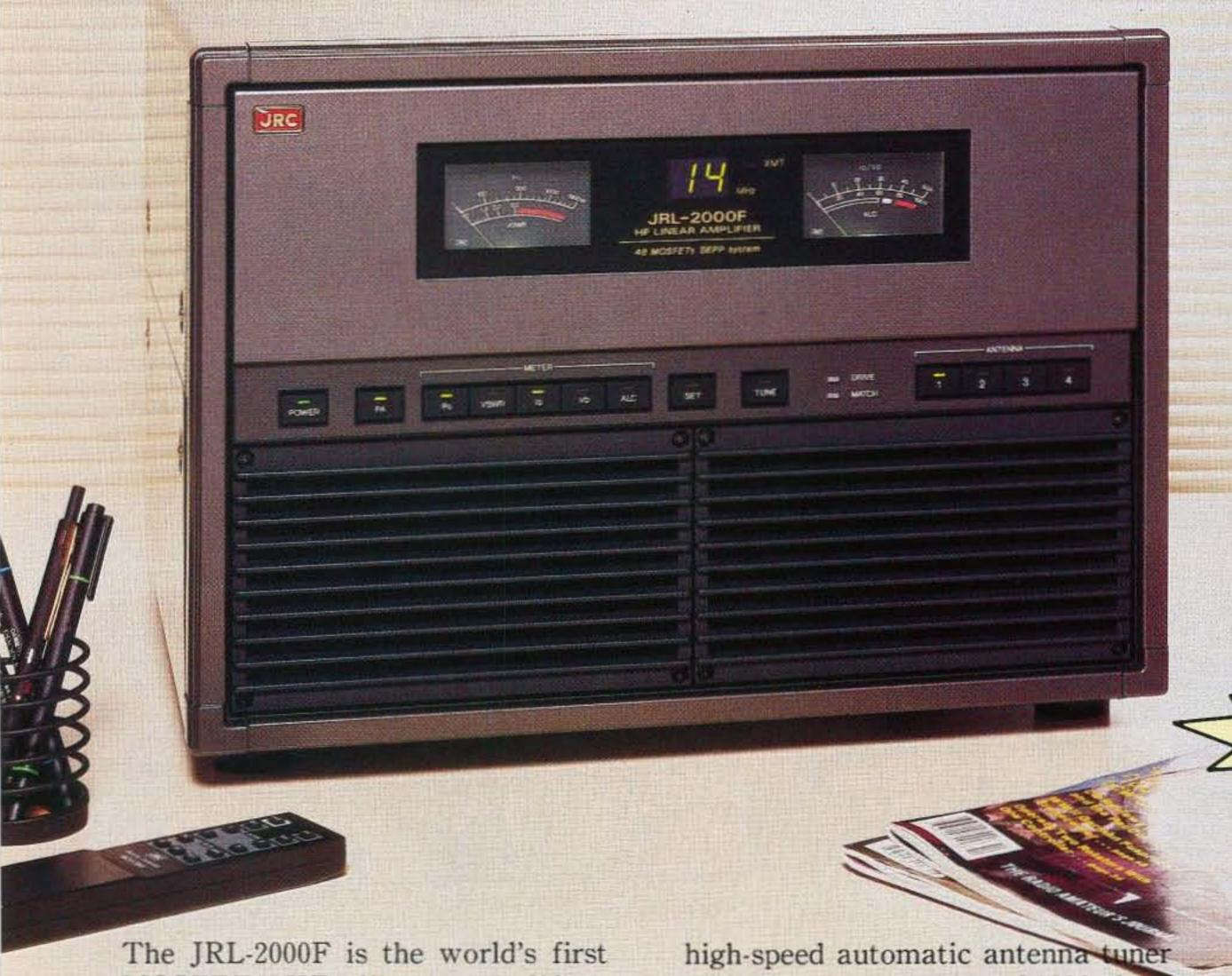
MOSFET HF linear amplifier, designed using the same high technology found in JRC's professional high-power radio transmitters. Featuring a heavy-duty power amp that incorporates 48 RF power MOS-FETs to ensure low distortion and clean output up to 1,000 watts (100% duty cycle, 24 hour) SSB/CW, plus a
